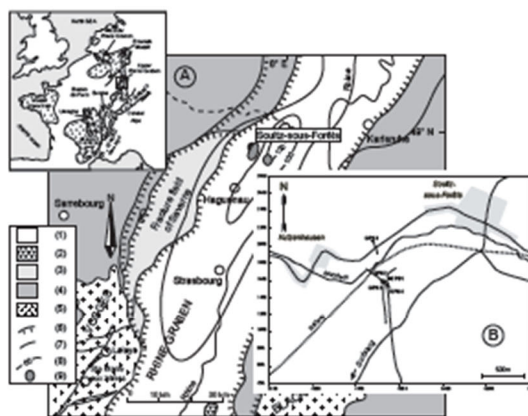
Figure 1. Location of the EGS Soutz site and geology of the Upper Rhine Graben. A: (1) Cenozoic sediments (2) Cenozoic volcanism (3) Jurassic (4) Trias (5) Hercynian basement (6) Boundary faults (7) Other faults (8) Temperature distribution in °C at 1500m depth (Haenel et al., 1979). (9) Local thermal anomalies (Haenel et al., 1979). B: Local map of the Soutz drill site with the well trajectories.
