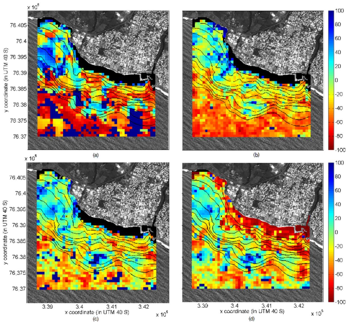
Fig. 4.5 11. Relative errors in bathymetry (in meters) on an **80 m × 80 m** grid from the SPOT-5 dataset for the following cases: (a) assuming a uniform wave period of **10.7 s** to compute the bathymetry, (b) using Fourier-filtered scenes and dominant waves only to compute the celerity, (c) using only dominant wave characteristics to compute the bathymetry, and (d) using all ( $\lambda, c$ ) clouds together to compute a single bathymetric value. The
