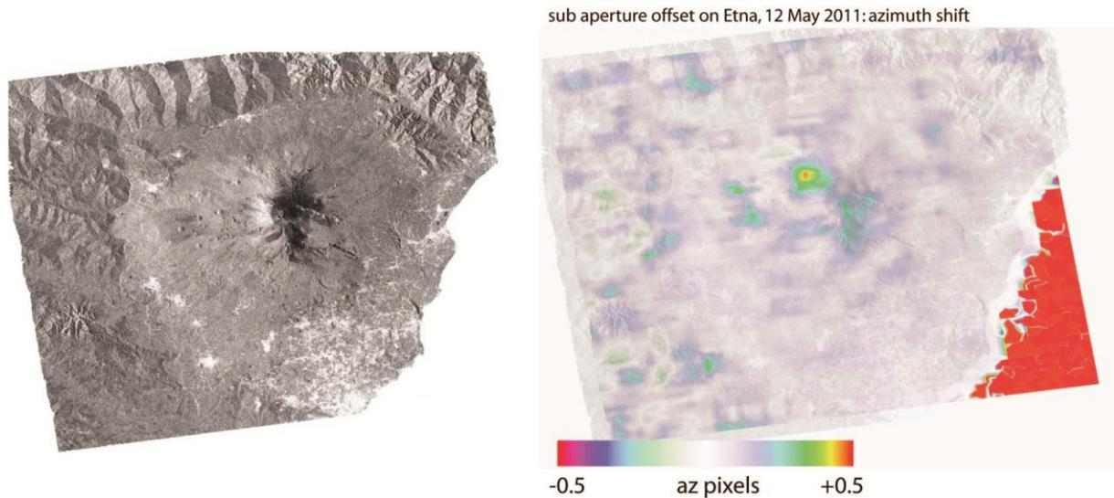
Figure 3.2.2 -1. Left, SAR amplitude image of Mount Etna. Right, SAR Doppler anomalies detected during the Etna volcano lava fountains episodes of 11 May 2011. Results published in the Aphorism project report (2016).
