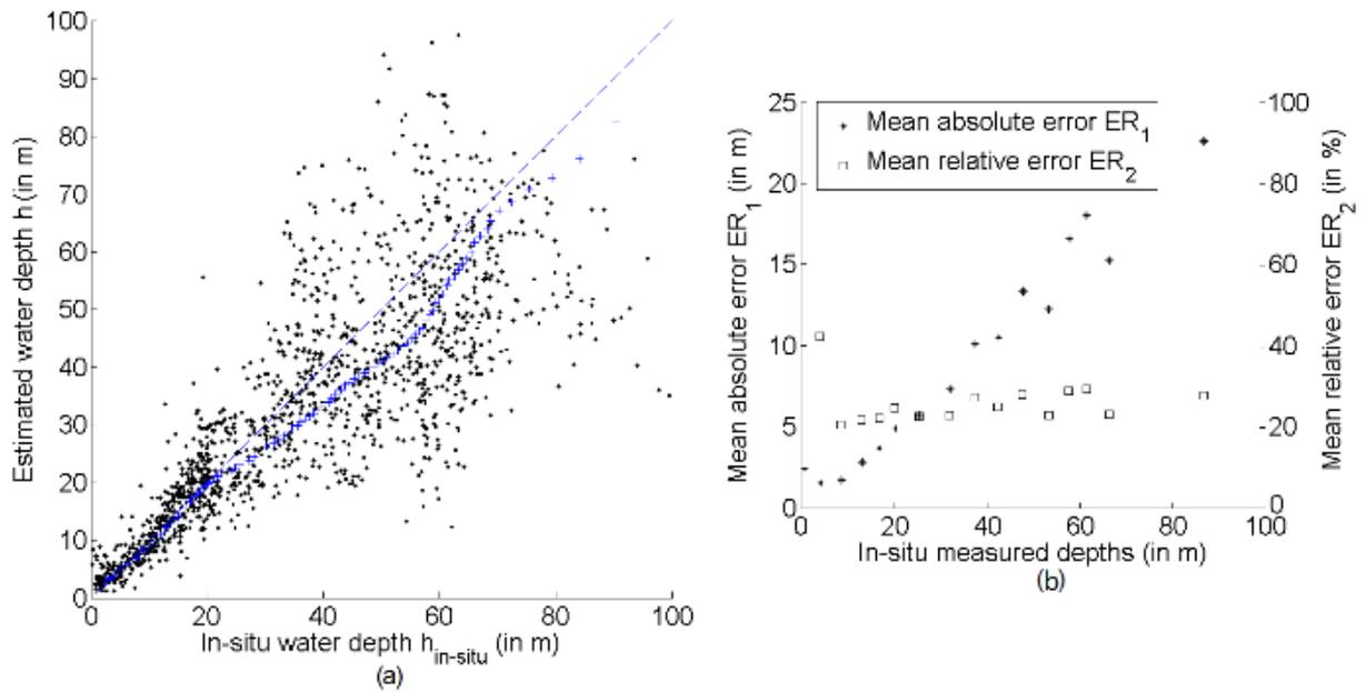
Fig. 10. (a) Water depths  $\hat{h}$  estimated from the satellite dataset versus *in-situ* measured water depths  $h_{in-situ}$  considering all the points of the **80 m × 80 m** grid. The blue crosses represent the 100 percentile ranks computed from  $h_{in-situ} = 2$  m. (b) absolute (\*) and relative (□) errors in bathymetry (in meters and in % respectively) for the 15 quantiles of *in-situ* measured depth.
