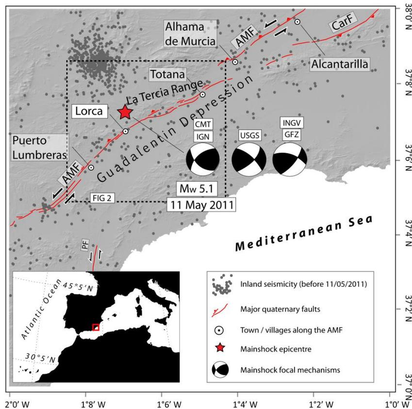
Figure 4.4 1. The study area. Locations of quaternary faults in red (after Martínez-Díaz (2002)). Seismicity recorded by IGN network before May 11, 2011, is shown in grey. The epicenter (red star) and the focal mechanisms of the main shock are as determined from the IGN moment tensor solution, INGV, GFZ and GCMT.
