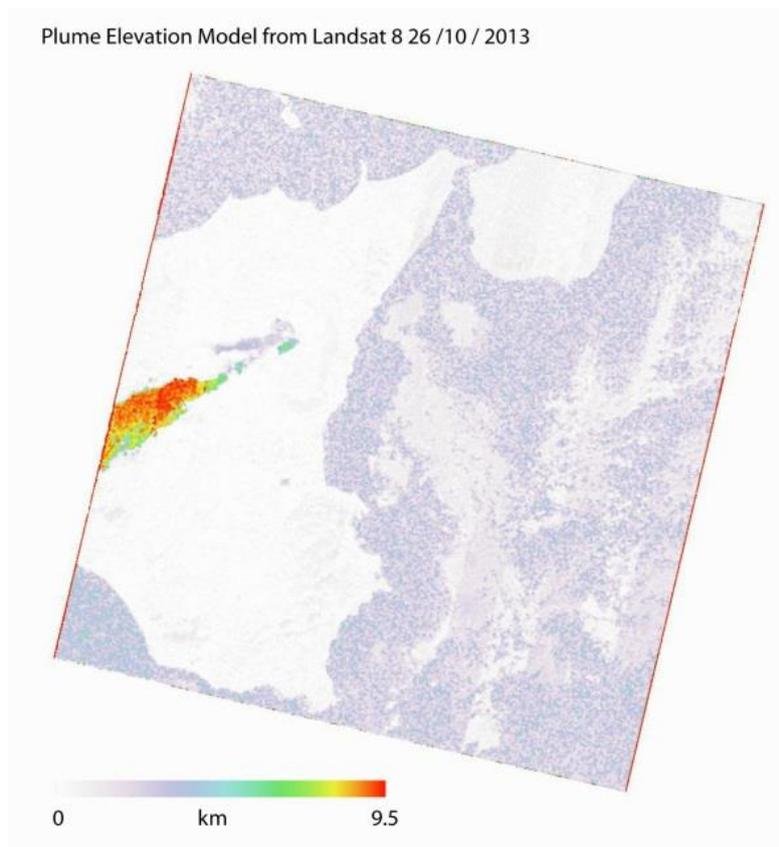
Figure 3.2.2 -2. Mount Etna eruption, 26 October 2013. Volcanic plume elevation form Landsat 8. Image © de Michele et al. 2015, BRGM (unpublished).
