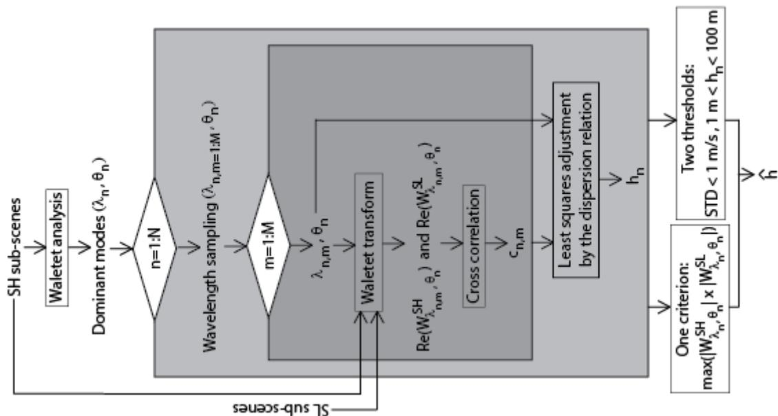
Fig. 4.5 1. Flowchart of the CWB methodology for retrieving bathymetry from two satellite images (**SH** for higher-resolution image and **SL** for lower-resolution image).
