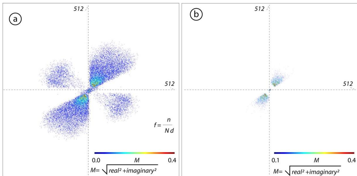
Figure 4.4 4. FFT spectrum calculated on a 512x512 pixels window over the ocean Image. A: FFT spectrum before the filtering. We can clearly see two preferential directions related to the swell (SW-NE) and the wind waves (SE-NW). B: FFT spectrum after filtering. We set the filter in such a way that FFT magnitudes less than 0.1 are discarded and only directions in the 1<sup>st</sup> and 3<sup>rd</sup> quadrant are retained for further processing.
