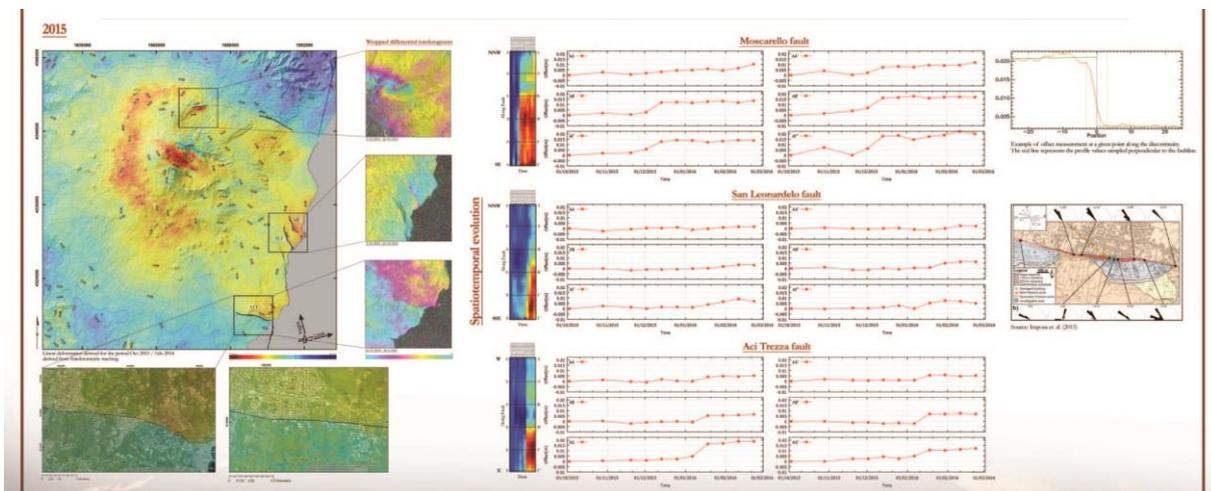
Figure 3.3 -2. Volcano deformation from Sentinel 1 interferometry. 2015 Etna eruption. Results presented at the MEDSUV final workshop 2016 as Derdelakos et al. (2016).
