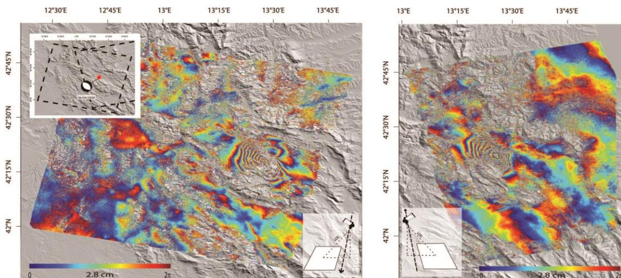
Figure 3.2.1 -1. The displacement field of the L'Aquila earthquake from C band ASAR Interferometry (ascending and descending modes). Image © de Michele et al. 2009, BRGM
