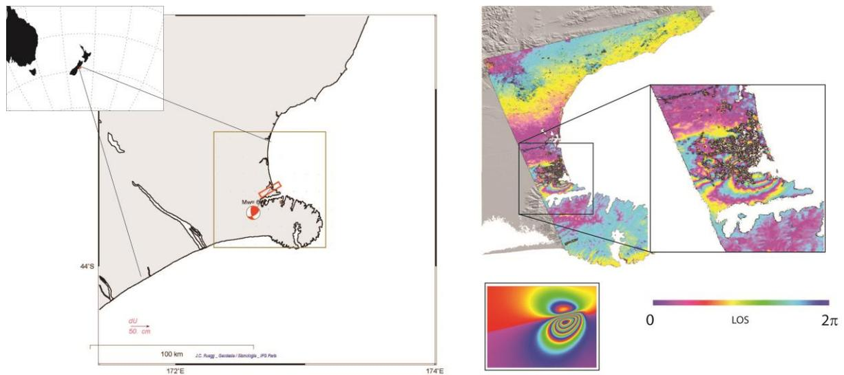
Figure 3.2.1 -2. The displacement field of the Christchurch earthquake as seen by ALOS PALSAR interferometry and elastic dislocation model. Image © de Michele et al. 2011, BRGM, ENS.
