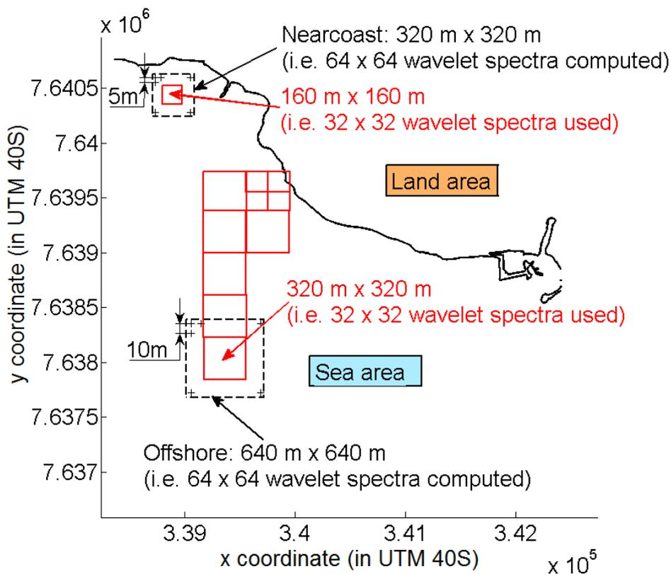
Fig. 4.5 7. Subscene dimension and resolution depending on distance from the coast.
