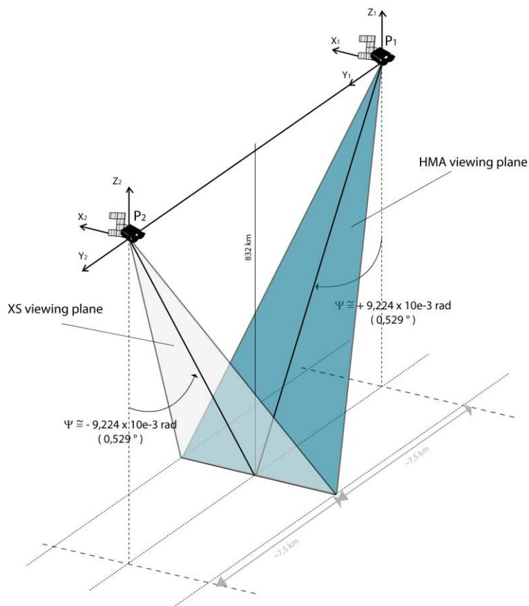
Figure 4.4 1. Acquisition geometry of SPOT5 HRG instrument (modified by the authors after Riazanoff, 2002 ). X, Y and Z represents the attitude state vectors stored in the ancillary data files; P1 and P2 indicate the position of the platform at  $T_0$  and  $T_0 + \Delta t$ , when acquiring the HMA and XS data respectively. In this case study,  $\Delta t = 2.04$  seconds.
