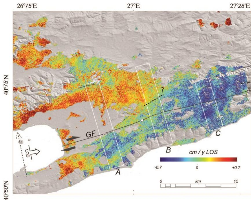
Figure 3.2.2 -3. InSAR PALSAR derived mean velocity on the Ganos section of the North Anatolian Fault zone.
