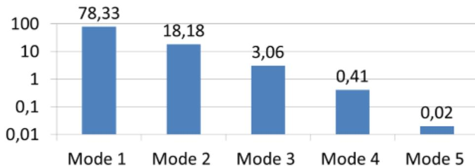
Fig. 4.5 8. Selection percentage of the modes. The modes are the maxima of spectral energy (Mode 1 (i.e.,  $n = 1$ ) being the most energetic and Mode 5 (i.e.,  $n = 5$ ) the least energetic).
