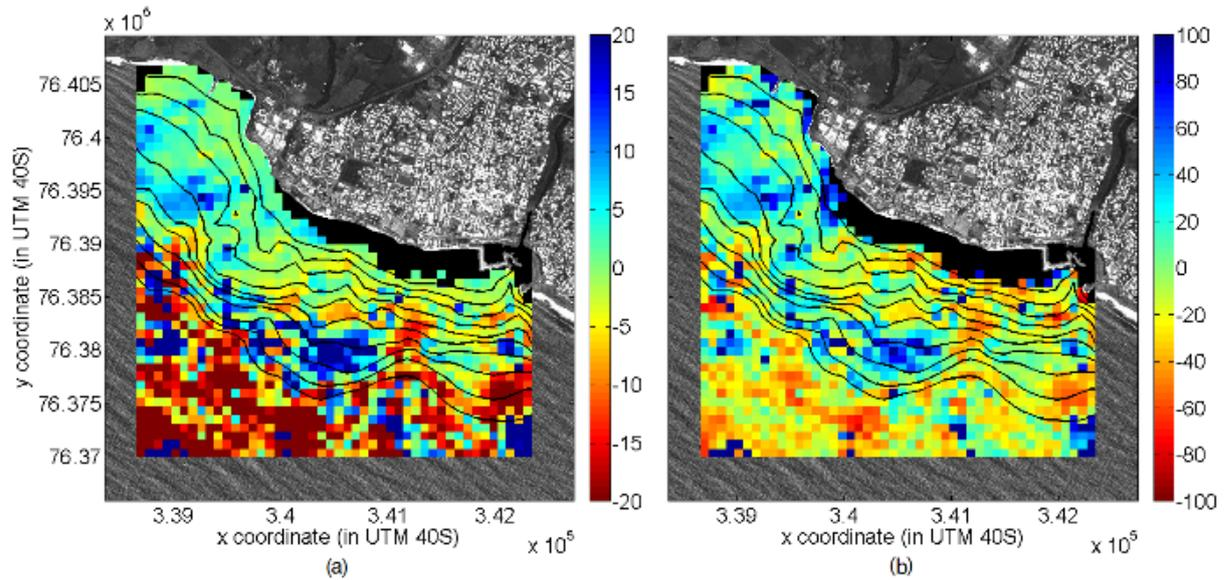
Fig. 4.5 9. Absolute (a) and relative (b) errors in bathymetry (in meters and in % respectively) on an  $80\text{ m} \times 80\text{ m}$  grid from the SPOT-5 dataset. The black curves represent the isobaths at each  $5\text{ m}$  until  $50\text{ m}$  given by the *in-situ* measurements. The black area near the coast is not covered by the method.
