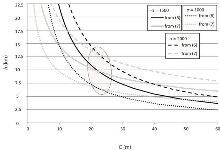
Figure 4.3 4. Plot of  $C$  (absolute path length in slant range) as a function of  $h$  (relative height of the source) from equations (4.3 6) and (4.3 7) we propose that the Doppler anomalous values can be compatible with a source located in between 6 and 12.5 km altitude, yielding an absolute wave path delay between  $\sim 19$  and  $\sim 25$  meters.
