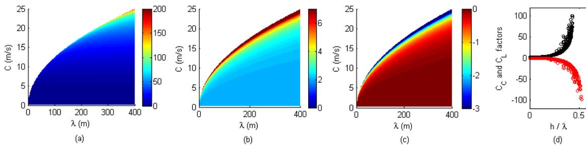
Fig. 4.5 12. (a) Theoretical water depth (in meters), (b) coefficient  $C_C$ , (c) coefficient  $C_L$ , (d) coefficients  $C_C$  (black) and  $C_L$  (red) versus water depth divided by wavelength, the linear dispersion being applicable for  $0.02 < h/\lambda < 0.5$ .
