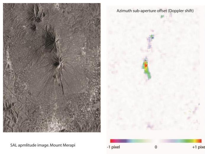
Figure 3.2.2 -4. Left, Radarsat amplitude image on mount Merapi on 23 November 2011. Right, sub-aperture offset indicating a Doppler anomaly during the SAR image acquisition process. In this very case, the Doppler anomaly might be due to lahars velocity. © de Michele et al. 2012, BRGM (unpublished).
