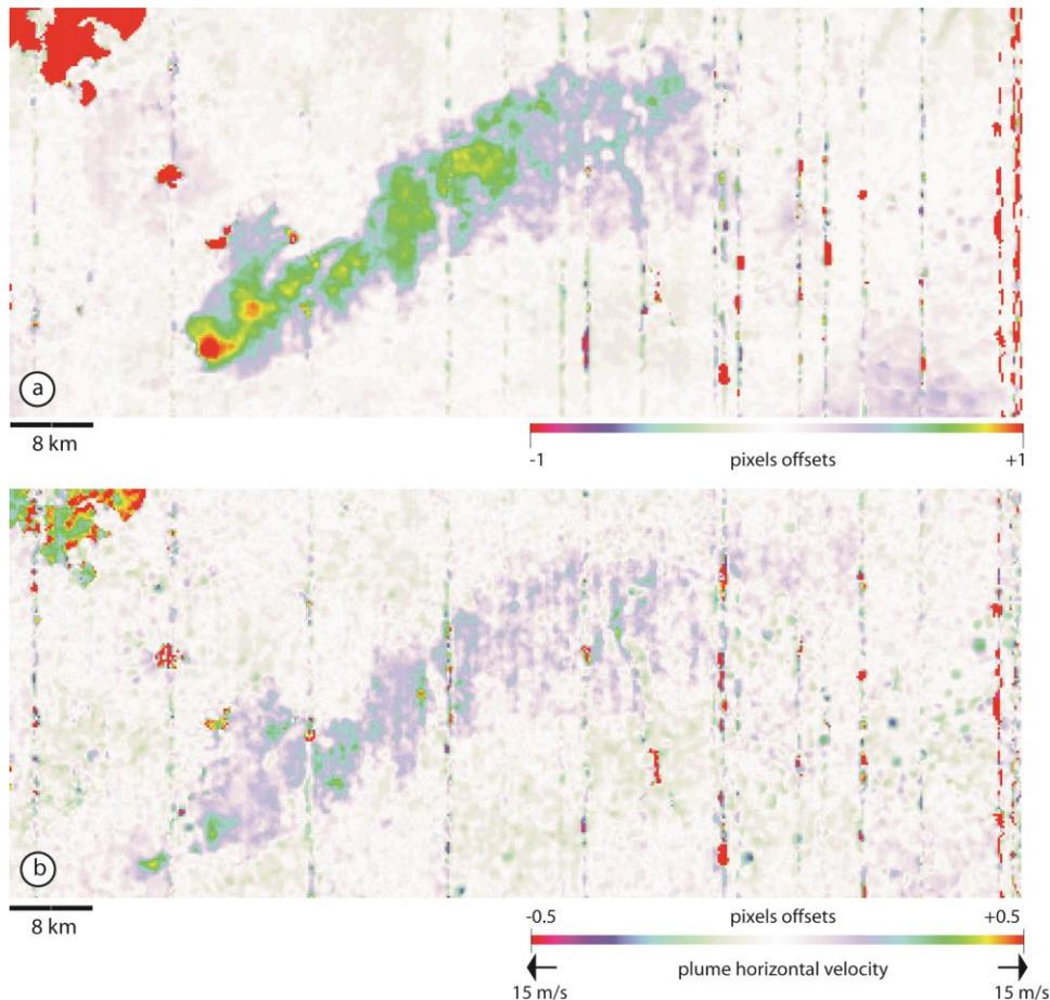
Figure 4.2 -2. Pixel offsets from correlation analysis. a) offsets in the epipolar direction due both to parallax and plume velocity in the along-track direction. b) P2E offset due to horizontal plume velocity in the P2E direction.
