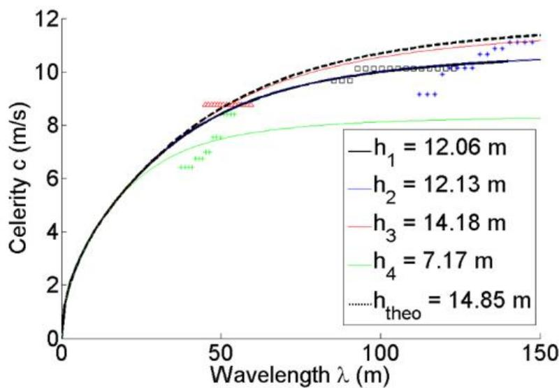
Fig. 4.5.2. Point clouds and nonlinear curve fitting corresponding to the  $n$  modes ( $n = 1$  (black),  $n = 2$  (blue),  $n = 3$  (red),  $n = 4$  (green)) at the P1 location (white cross on Fig. 3b). The selected  $\hat{h}$  is indicated with a thicker line (here, it is  $h_1$ ). The theoretical curve obtained using the in-situ bathymetry is shown by a dotted line.
