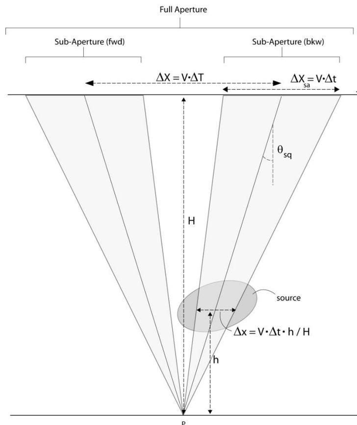
Figure 4.3 2: Geometry of the sub-aperture acquisition.  $\Delta T$  is the time separation between looks,  $\Delta t$  is the sub-aperture integration time,  $V$  is the along track velocity of the platform,  $\theta_{sq}$  the squint angle of the sub aperture
