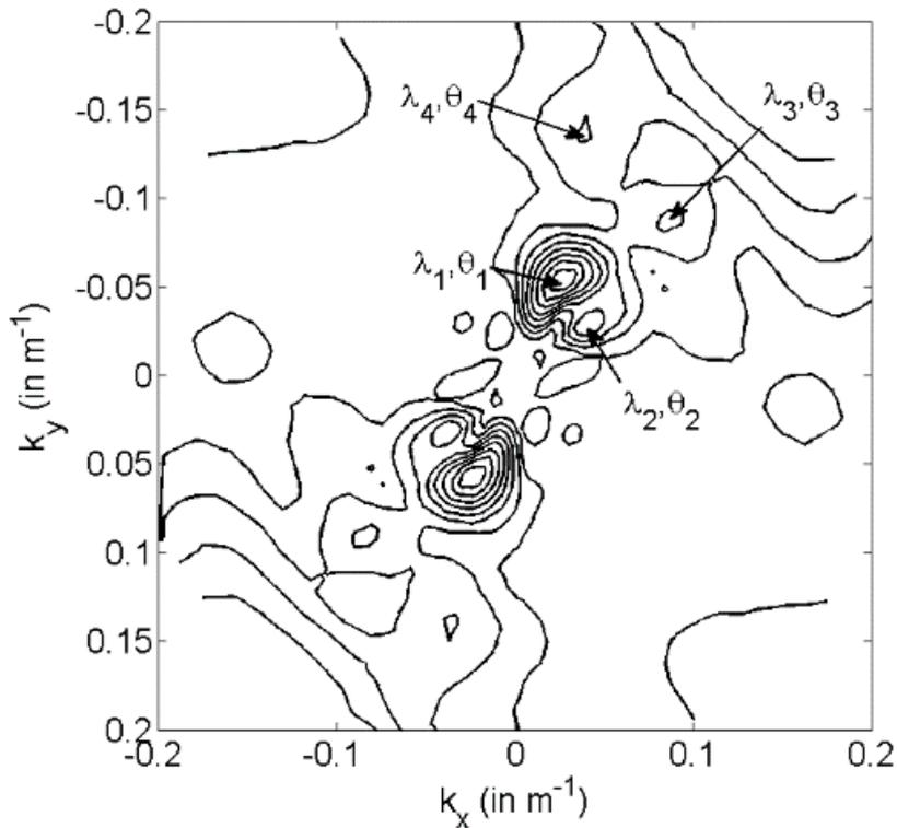
Fig. 4.5 4. Normalized wave amplitude spectrum  $W_{\bar{x}}$  at the P1 location (white cross in Fig. 3b). The spectrum is expressed in terms of wave number in the  $(k_x, k_y)$  plane using the following convention:  $k_x = 2\pi \sin(\theta)/\lambda$  and  $k_y = 2\pi \cos(\theta)/\lambda$ . The dimensionless maximum spectral intensity is  $W_{\bar{x}} = 0.1$ , and the contour intervals are **0.01**.
