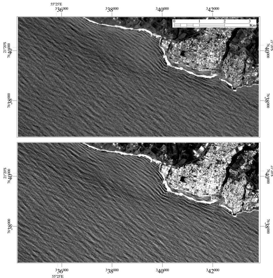
Figure 4.4 3. SPOT5 HRG dataset, south of La Reunion Island. Top: the HMA image (subsamped to the 10 m resolution XS image). Bottom: the XS image. We can observe a signal due to the SW/NE swell as well as a higher frequency wind waves directing SE-NW.
