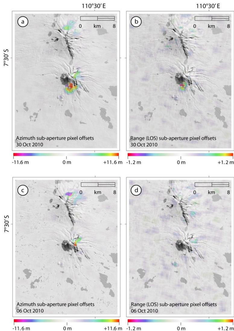
Figure 4.3 3. Pixel offsets measured by sub-aperture cross correlation calculated on the SAR data acquired on the 30 of October 2010 during the Merapi volcano eruption; a) azimuth direction, b) range direction. Apparent pixel offsets measured by sub-aperture cross correlation calculated on the SAR data acquired on the 06 of October 2010, before the Merapi volcano eruption; c) azimuth direction, d) range direction.
