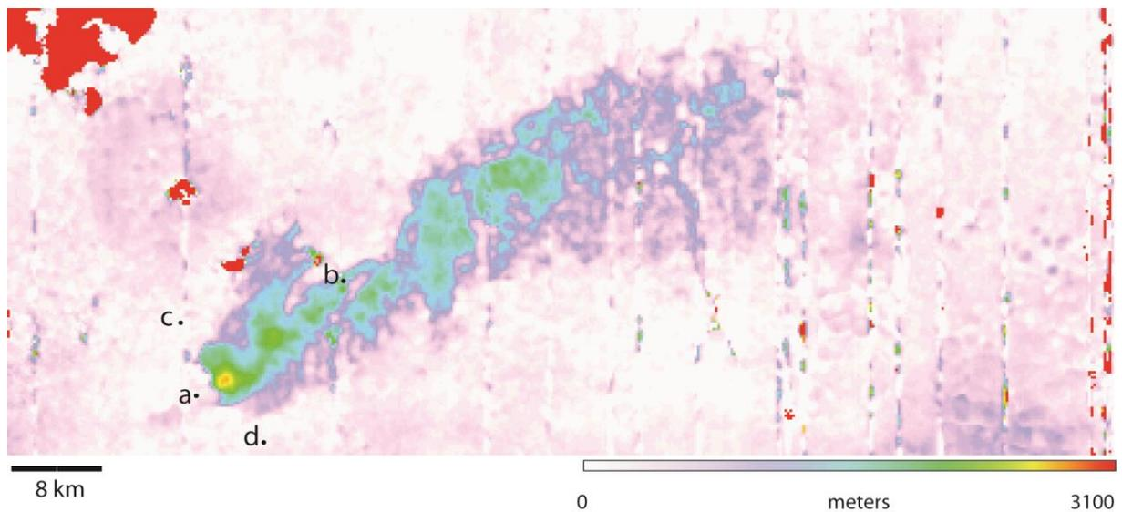
Figure 4.2 -3. The Holuhraun Plume Elevation Model on 6 September 2014 with a spatial resolution of 240 m per pixel. Location of the a-b and c-d elevation profiles in Fig. 4.2 -4 are shown.
