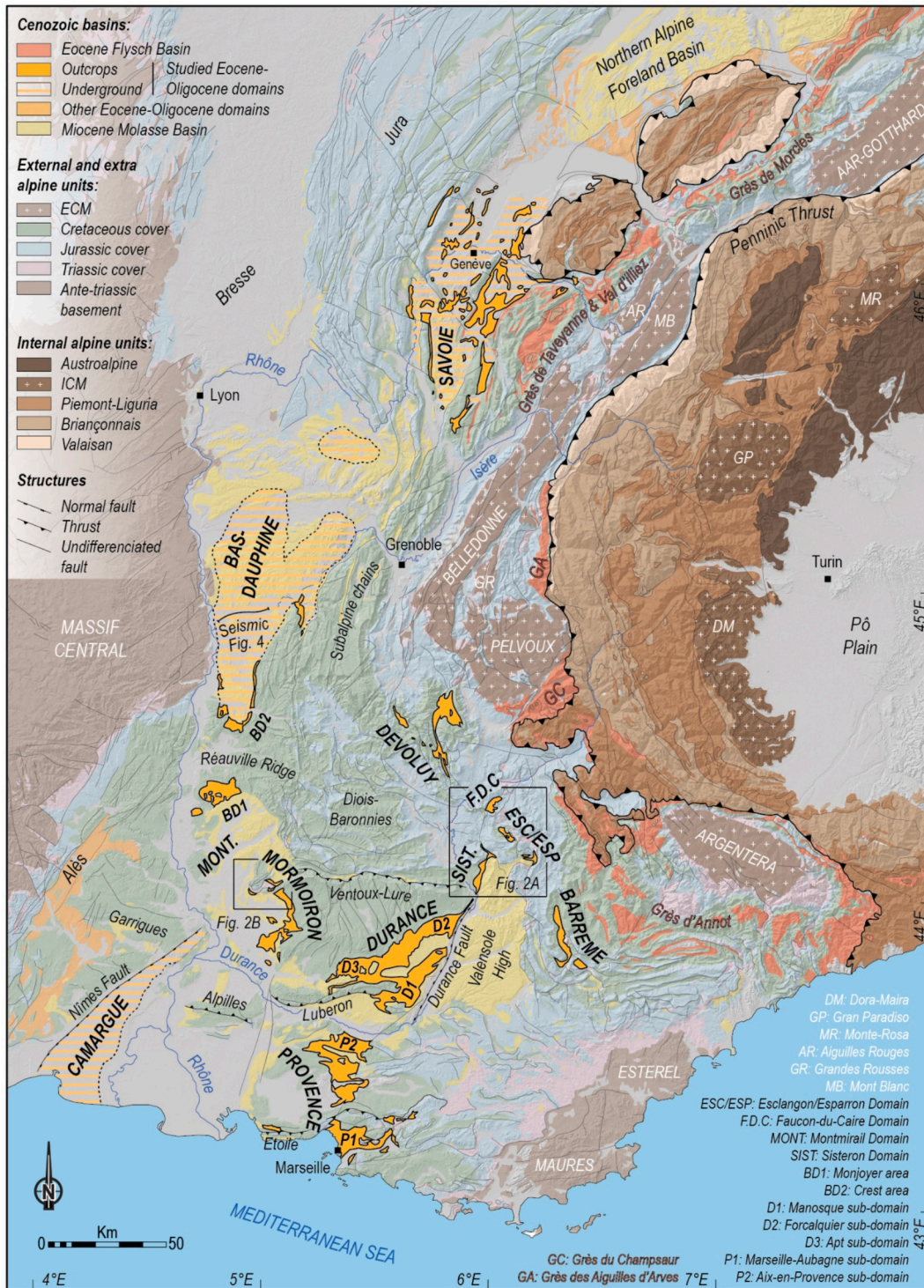
Fig. 1. Geological map with superimposed shaded relief of the western Alps and the WAFB adapted from the geological map of Bureau de recherches géologiques et minières (1/1000000; https://infoterre.brgm.fr/ ).
