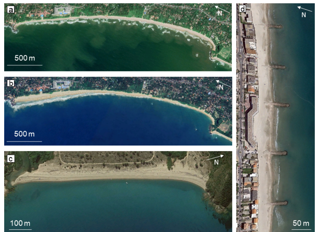
Figure 1. Examples of embayed beach planforms. (a,b) Asymmetric curved beach showing large change in shoreline orientation between (a) November 2021 and (b) February 2024 due to embayment rotation at Balapitiya beach, Sri Lanka; (c) straight shoreline between natural headlands at Porto-Vecchio, France; (d) straight shoreline between artificial groynes at Palavas-les-flots, France. Images adapted from Google Earth.
