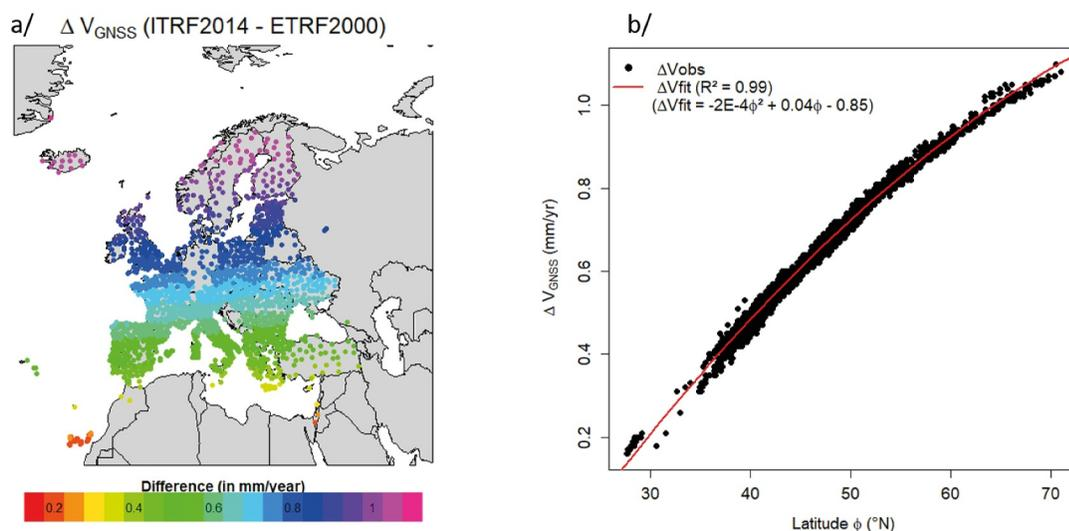
**Figure 3.** Analysis of EPN global navigation satellite systems vertical velocity differences in the ITRF2014 and ETRF2000 geodetic reference frames in Europe. (a) European mapping of the vertical land velocity differences. (b) Vertical land velocity difference as a function of the latitude.
