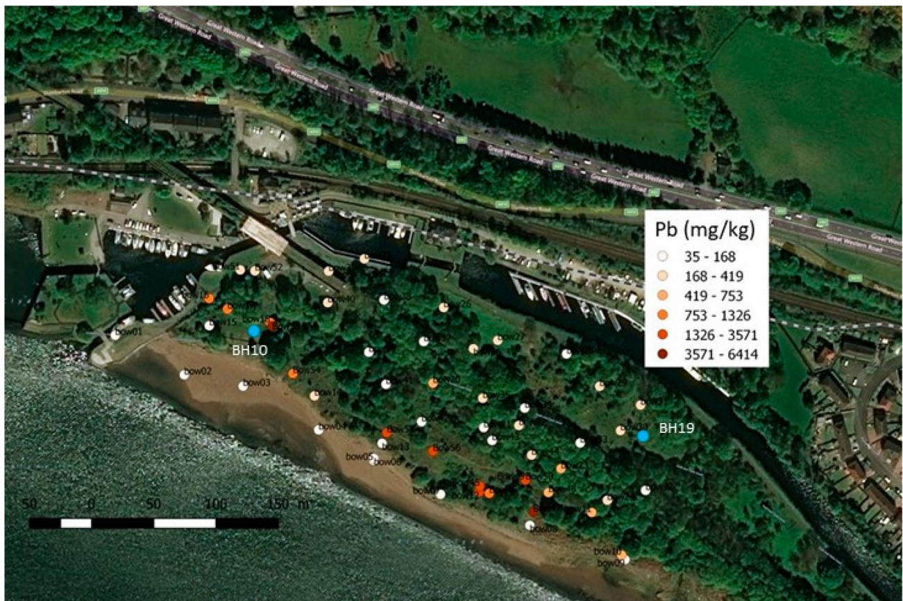
Fig. 8 Lead (Pb) measurements by pXRF in soil at the canalside regeneration area at Bowling (from: Lemiere et al. 2022)
