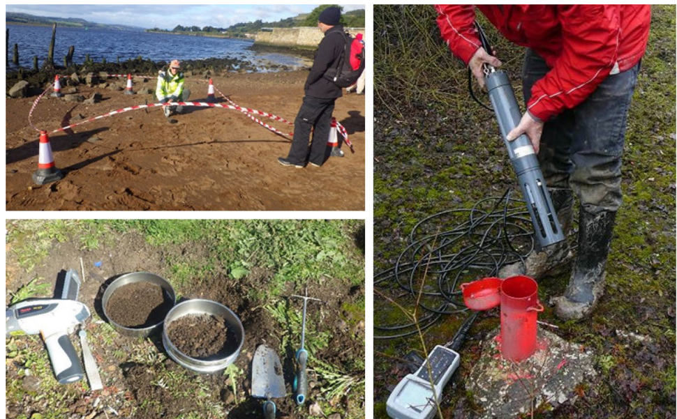
Fig. 3 On site monitoring of sediment chemical characteristics with a handheld XRF (left) and groundwater quality (right) by multiparametric probe at the Bowling site, Scotland, UK (from: Lemier et al. 2022)
