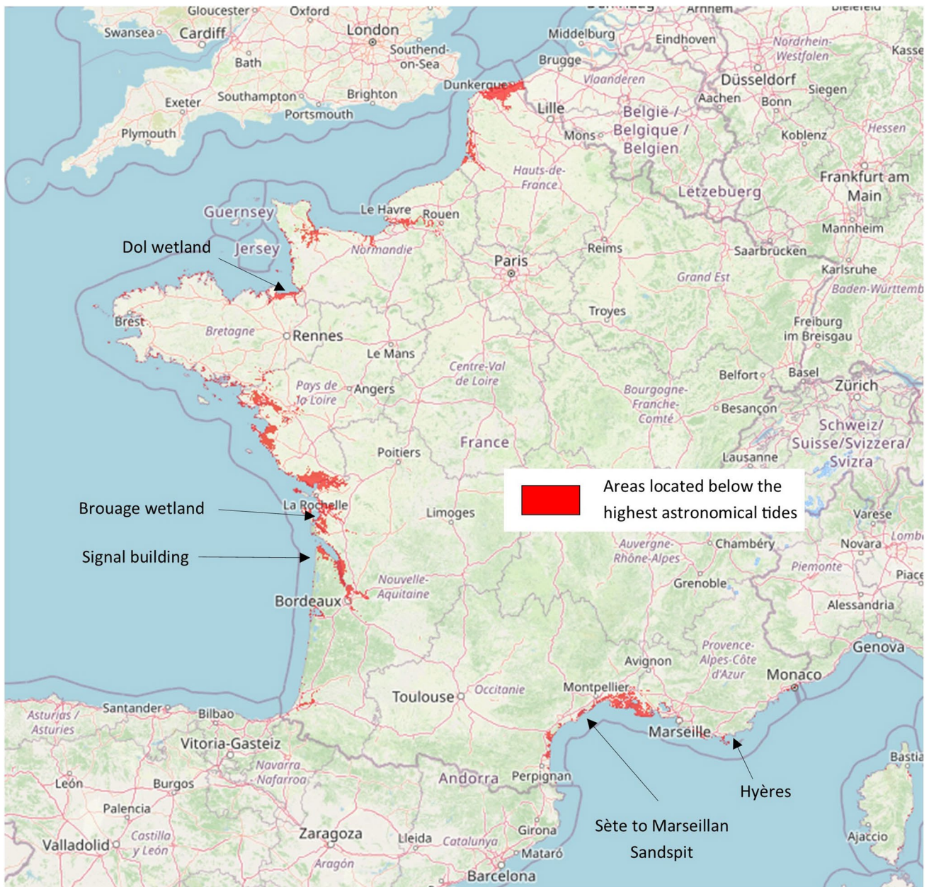
Fig. 5 Map of mainland France showing areas located below the highest astronomical tides today. These areas are not flooded due to natural and man-made protections. Data: IGN (Lidar topography),
