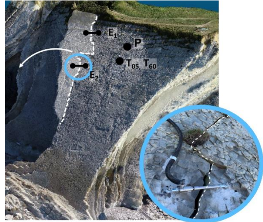
Figure 1: Experimental set up with extensometers (E), Pyranometer (P) and Temperature probes (T). The instable slab (white) is supposed to have a rotational movement. Inside the blue circle: photo of one extensometer across the joint (dashed line)
