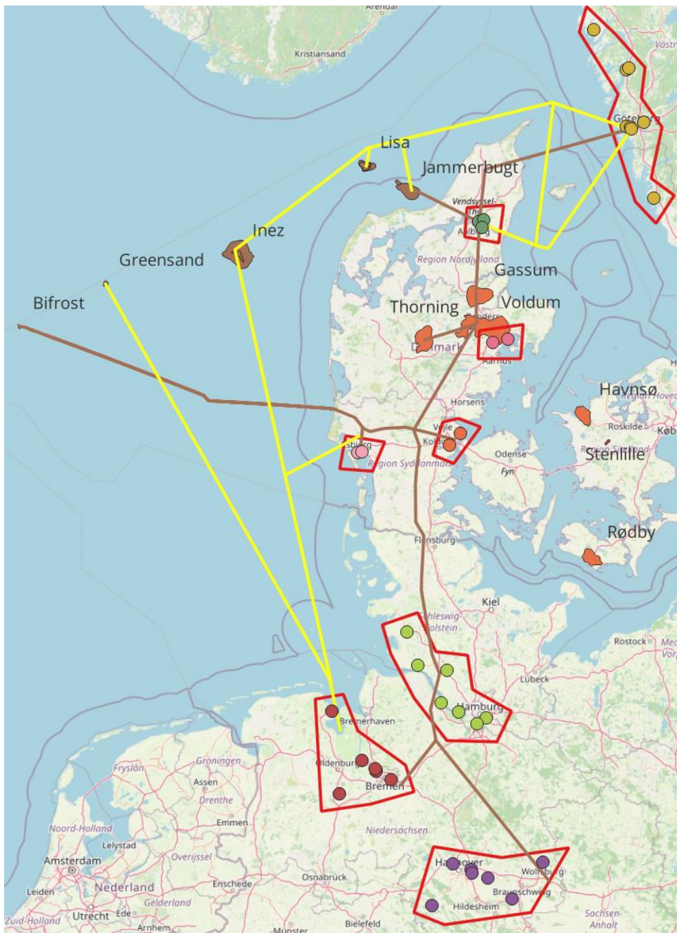
Figure 4.33: Jutland value chain. Dots surrounded by red polygons represent emission clusters. Orange and brown forms represent onshore and offshore storage sites, respectively. Yellow and brown lines represent shipping and pipeline transportation, respectively.
