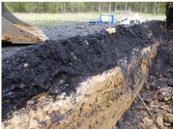
“Place à Gaz” chemical ammunition BG near VERDUN. Cross section made by excavation showing a 40 cm thick black layer of OB residue. 200,000 chemical “Blue-Cross” shells have been burned on this spot around 1926 by the company FN PICKETT & Fils.
