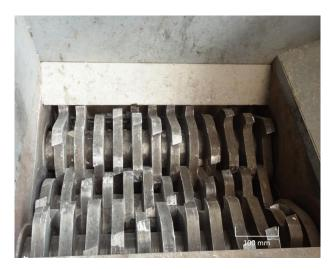
Figure 2. Inside view of the shredder DECOVAL 3K7/30.
