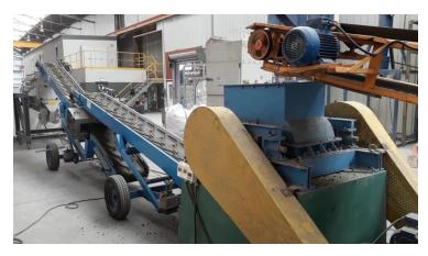
Figure 13. Step of toothed roll crushing with 10 mm sieve directly connected (in the back).
