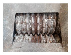
Figure 4. Inside view of the toothed roll crusher.
