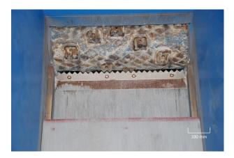
Figure 3. Inside view of the single roll shredder (top: toothed cylinder, bottom: push-piece).
