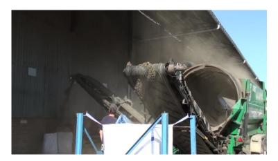
Figure 12. Step of rotating drum sieving.
