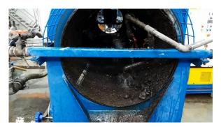
Figure 15. Separation of coarse materials in the rotating drum (trommel).
