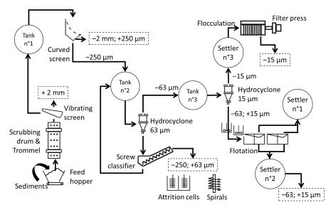
**Figure 6.** General scheme of the SOLINDUS pilot platform.
