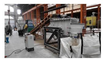
**Figure 14.** Step of fluted roll crushing (in the back) with the 10 mm sieve directly connected (in the front).
