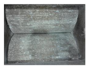
**Figure 5.** Inside view of the fluted roll crusher.
