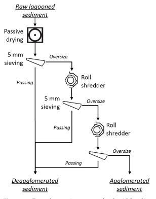
Figure 10. Deagglomeration process for the ALS sediment.
