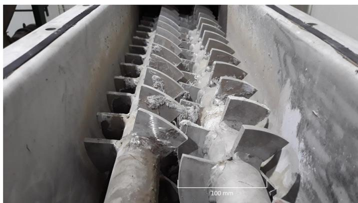
**Figure 1.** Inside view of the screw feeder SOFRADEN MPS120.
