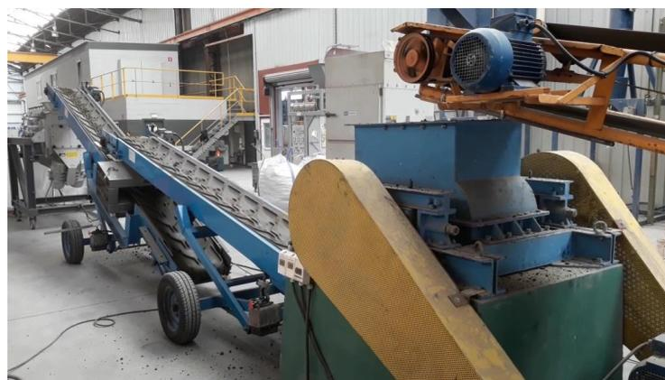
**Figure 13.** Step of toothed roll crushing with 10 mm sieve directly connected (in the back).
