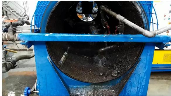
Figure 15. Separation of coarse materials in the rotating drum (trommel).
