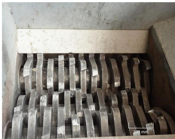
**Figure 2.** Inside view of the shredder DECOVAL 3K7/30.
