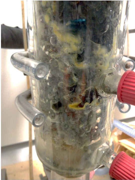
Bottom of the column bioreactor At the end of experiment
