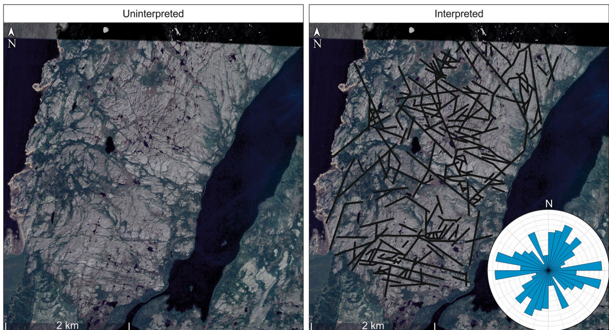
Fig. 3 Google Earth satellite image and rose diagram produced from structural lineament interpretation
