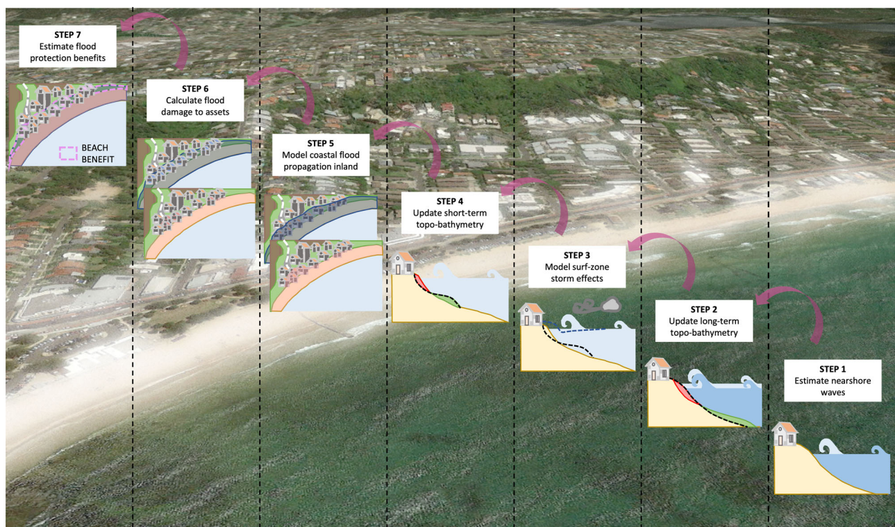
Fig. 1 | Key steps for estimating the flood protection services provided by beaches. From right to left. Step 1: Nearshore wave downscaling. Step 2: Integration of erosion on topo-bathymetries due to sea-level rise. Step 3: Modelling of surf-zone morphodynamics and hydrodynamics. Step 4: Integration of storm erosion on
