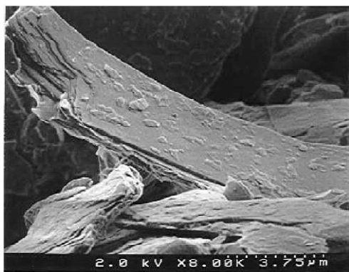
Fig. 1. Observation of talc 1 using SEM.
