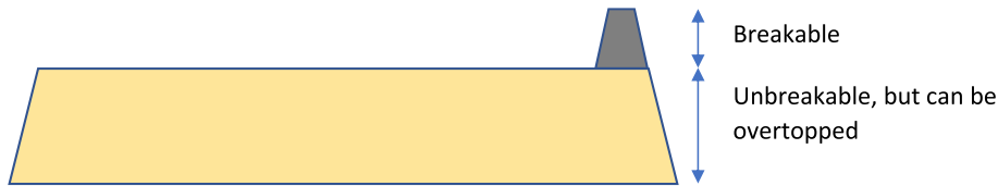
Fig. 2. Illustration of an artificial island with a flood defence.
