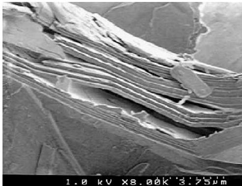
Photo 1. Microscopic porosity of a delaminated particle.
