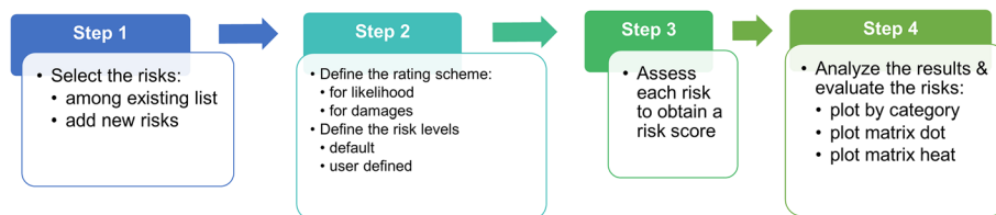
Fig. 1 Steps to perform to realize a risk analysis with the risk register tool. Each step corresponds to a different tab in the tool
