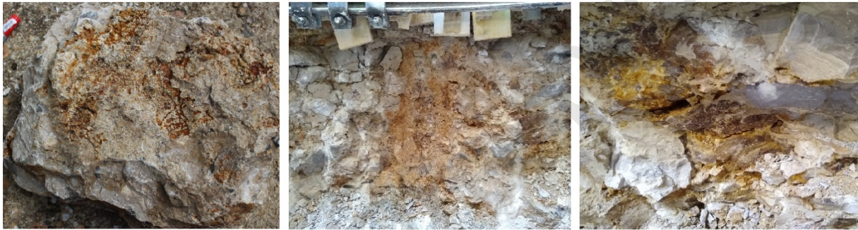
Fig. 7. Images of the altered and fissured limestone formation taken while drilling the main well at the O-ZNS observatory.
