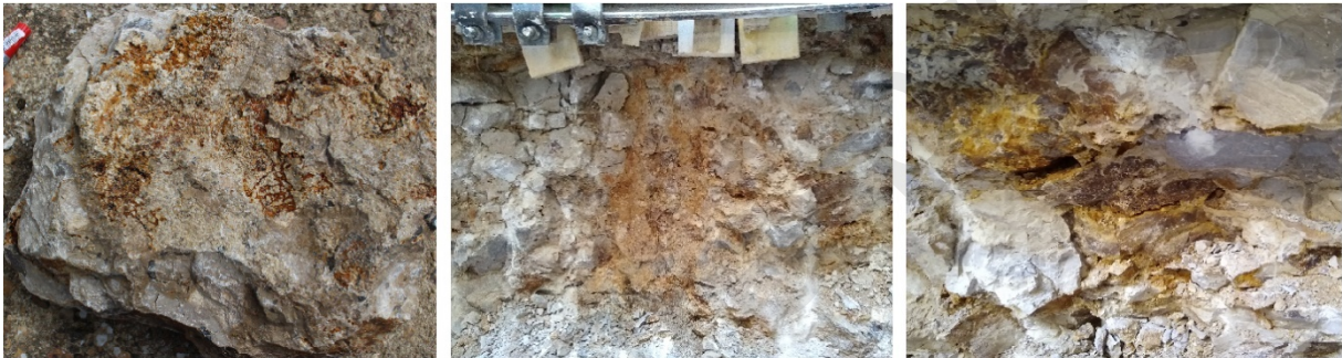
469 470 Fig. 7. Images of the altered and fissured limestone formation taken while drilling the main 471 well at the O-ZNS observatory.
