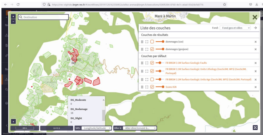
Fig. 13 Visualization through the User Web portal of VIGIRISKS of the damage results for mapping deformation of slow landslides in La Reunion
