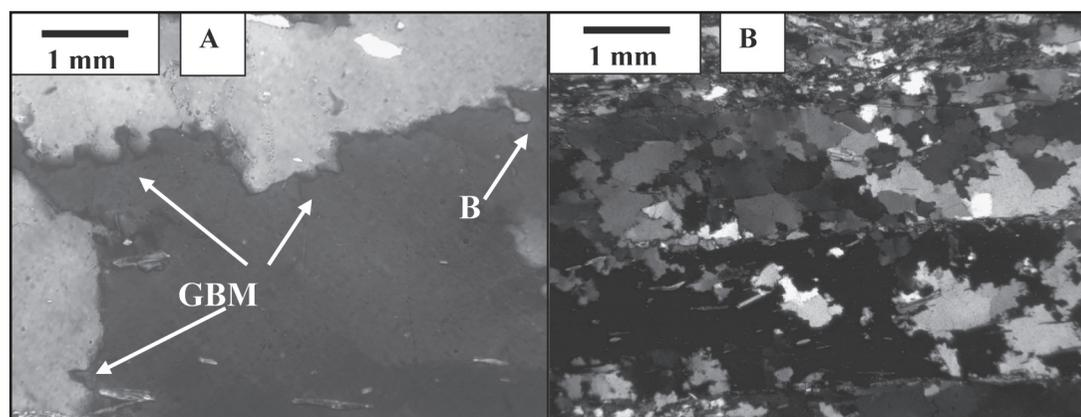
**Fig. 8:** Cross-polarized-light view of PLAR 70 showing foliation and quartz texture indicating important quartz grain boundary migration. **A:** Enlargement showing evidence of grain boundary migration (GBM) and bulging (B).
