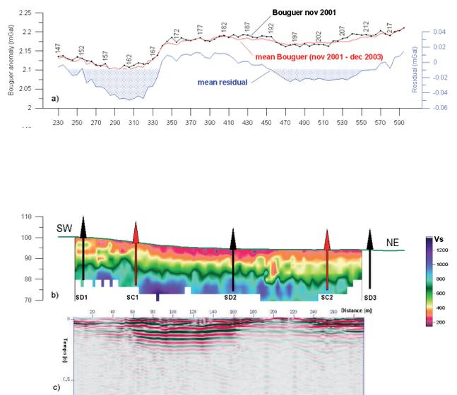
FIGURE 9 High-resolution MASW and microgravity reconnaissance along the central part of Profile 3: (a) gravity anomalies; (b)  $V_s$  velocity section; (c) surface-wave image stack.
