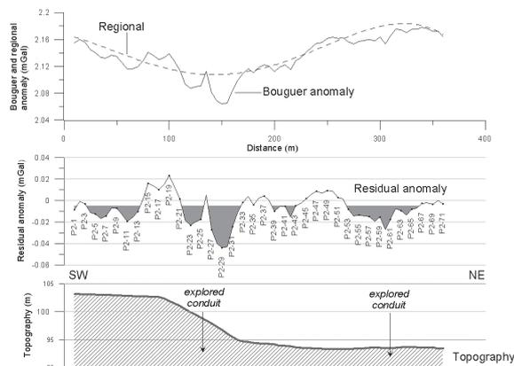
FIGURE 6 Profile 2: Bouguer anomaly, residual anomaly and topography with location of explored conduits.
