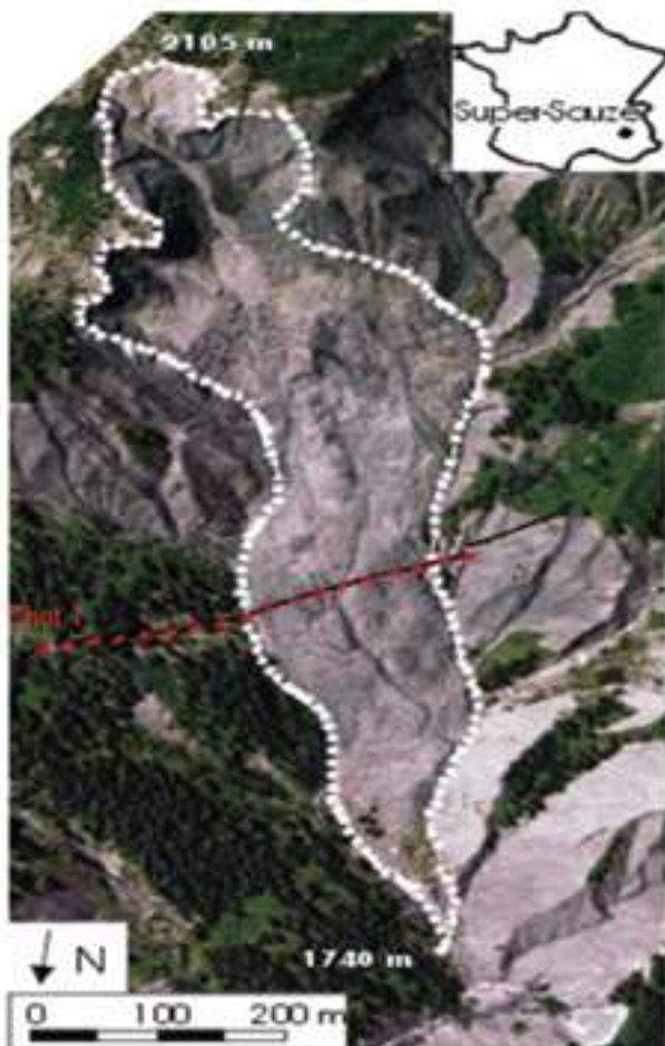
FIGURE 1 Location of Super-Sauze earthflow showing the seismic line; red stars indicate sources, black points indicate receivers.
