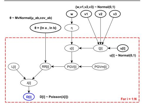
Fig. 4 Bayesian model implemented in OpenBUGS. Bold nodes represent stochastic variables, with their prior distributions. The blue node represents the damage variable evidenced from field observations
