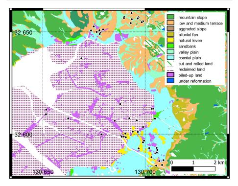
Fig. 9 Detailed soil condition map for the central part of Uki City. The black dots represent the 50 damage locations that have been observed. Soil condition data by GSI (2013)
