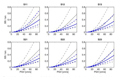
**Fig. 6** Median and 16–84th percentile RR functions obtained from the Bayesian model (solid and dashed blue lines), for each of the six shake-maps. The grey lines represent the prior distribution, obtained from the selection of existing RR functions
