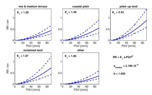
Fig. 10 Median and 16-84th percentile RR functions obtained by discriminating different soil conditions
