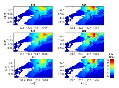
Fig. 2 PGV shake-maps derived using the different assumptions on fault geometry and GMPEs
