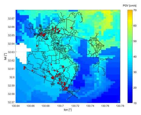
Fig. 3 Layout of the main part of the water supply network (solid black lines), with the observed damage locations (red diamonds). The underlying PGV distribution is based on shake-map S11
