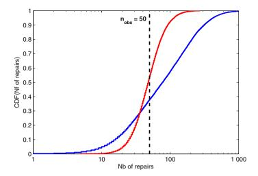
Fig. 12 Empirical CDF of loss metric M<sub>1</sub>, for both cases #1 (in blue) and #2 (in red)
