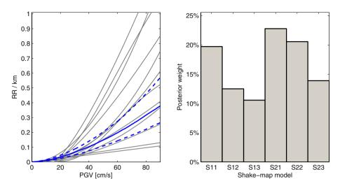
Fig.8 Left: Updated RR function (solid and dashed blue lines) accounting for the different shake-maps, and prior existing RR functions (grey lines); Right: Posterior distribution of categorical variable S (i.e. weight of each shake-map in the sampling)
