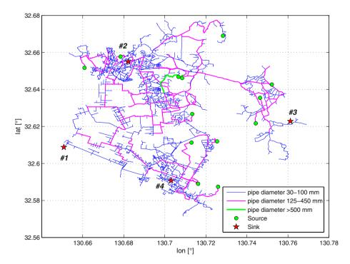
Fig. 11 Layout of the water supply network with the sources (reservoir tanks, green circles) and four sinks (distribution points, red stars)
