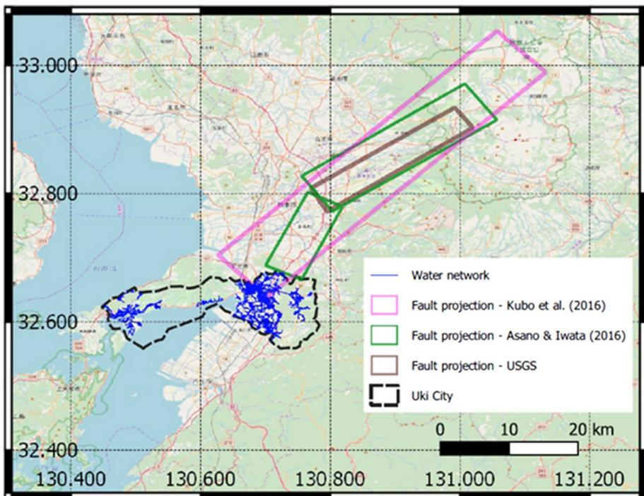
**Fig. 1** Situation of Uki City and of the water supply network with respect to the projected faulting of the  $M_w$  7.0 Kumamoto earthquake main-shock (three different fault geometries considered)
