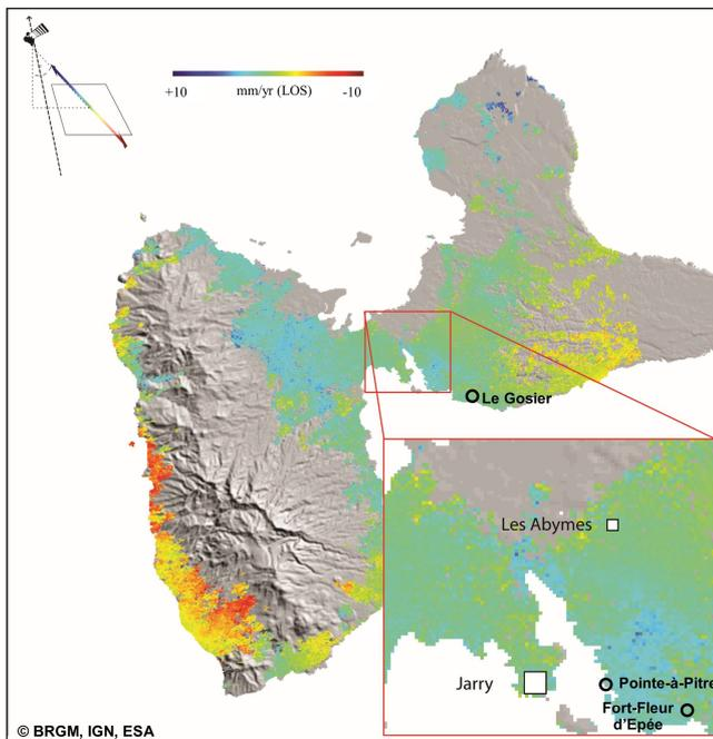
**Figure 4.** Linear velocity map from the multi baseline InSAR method. These results are based on the analysis of 34 radar scenes acquired between 2003 and 2010 by the ASAR sensor on Envisat of the European Space Agency (map created by BRGM; data: IGN, ESA; © BRGM, IGN, ESA).
