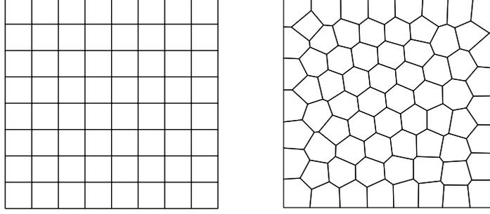
Figure 1: Cartesian and Voronoi meshes for the numerical tests.
