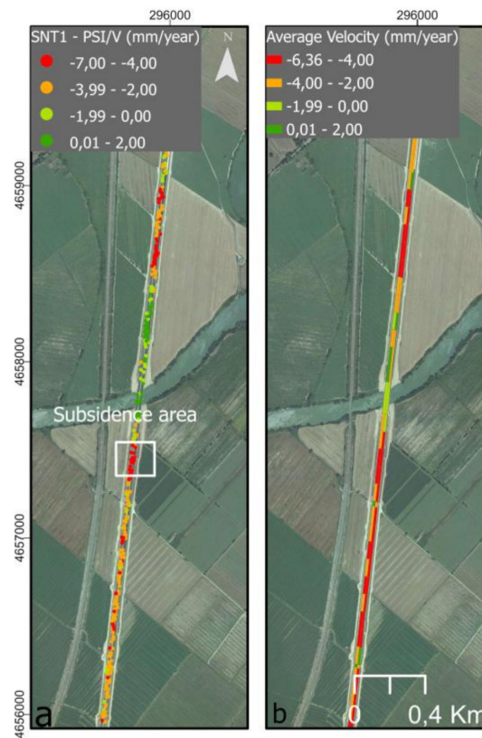
Figure 5. (a) Displacement map PSI Sentinel-1 for D18 highway, (b) Map classification section average velocity (mm/year), as background orthophoto Rome.
