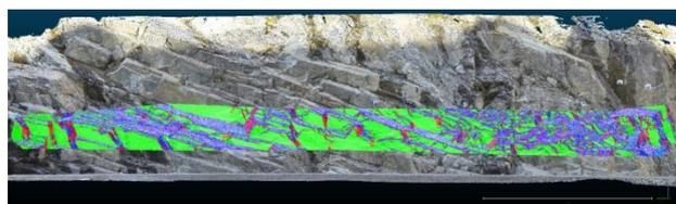
Figure 2. 3D RGB point cloud with a 1m-high area of interest around the scan line survey where normal are colored by HSV.
