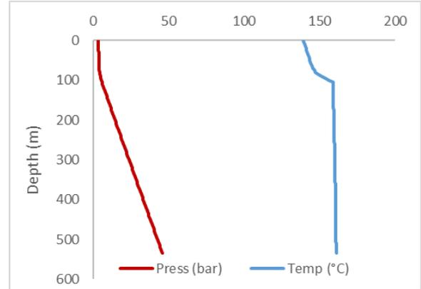
**Fig. 4: The pressure (in red) and temperature (in blue) profiles in the geothermal well #2.**
