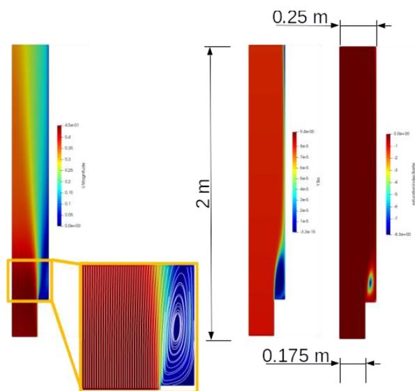
**Fig. 6: Left: flow profile in the well where the cross-section expands with vortices developed at the corners of the expanding cross-section of the well. Right: Barium concentration profile and barite saturation index**
