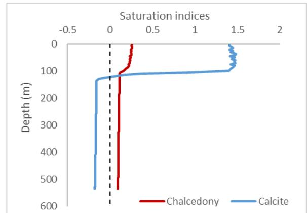
**Fig. 5: The saturation index profile for minerals – calcite (in blue) and chalcedony (in red) in the geothermal well #2. The dashed black line indicates equilibrium (saturation index of 0) for reference.**
