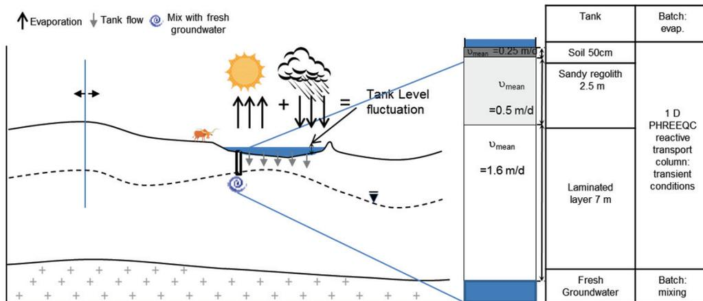
Fig. 2. Conceptual model of hard-rock aquifer in southern India with Managed Aquifer Recharge (MAR) through an infiltration tank used for the development of a 1D Phreeqc reactive column model.  $v_{mean}$  is the mean pore flow velocity.
