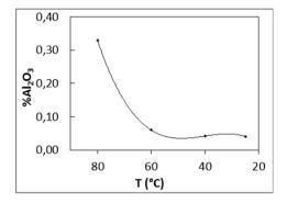
Fig. 9. Evolution of %Al<sub>2</sub>O<sub>3</sub>as function oftemperature
