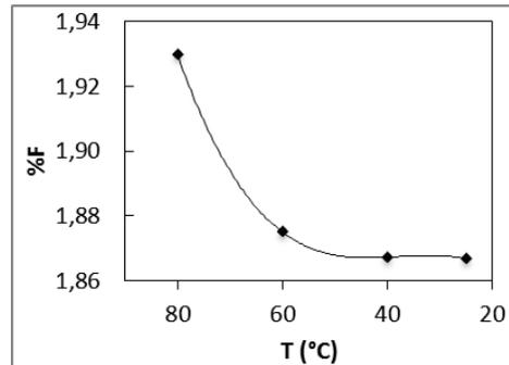
Fig. 4. Evolution of %F (fluoride) as function of temperature
