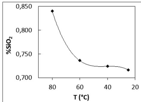
Fig. 5. Evolution of %SiO<sub>2</sub> as function of temperature
