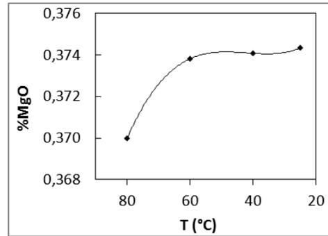
Fig. 8. Evolution of %MgO as function of temperature.
