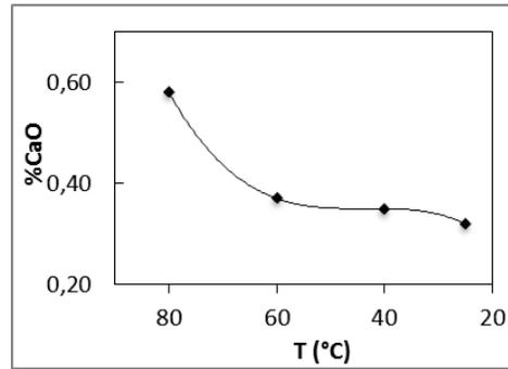
Fig. 2. Evolution of %CaO as function of temperature
