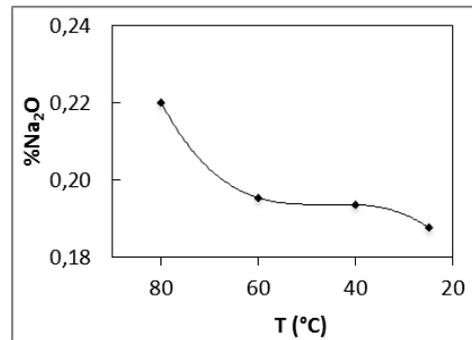
Fig. 6. Evolution of %Na<sub>2</sub>O as function of temperature
