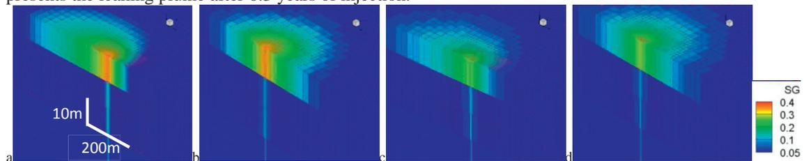
Figure 5: overlying aquifer after 6.3 years of injection in the main aquifer – a) 1m/y gw flow + lower  $P_{cap}$ , b) no gw flow + lower  $P_{cap}$ , c) 1m/y gw flow + higher  $P_{cap}$ , d) no gw flow + higher  $P_{cap}$
