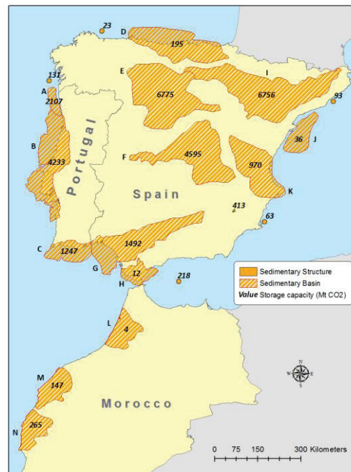
Figure 4. Location of potential storage areas and their estimated capacities in the West Mediterranean region.
