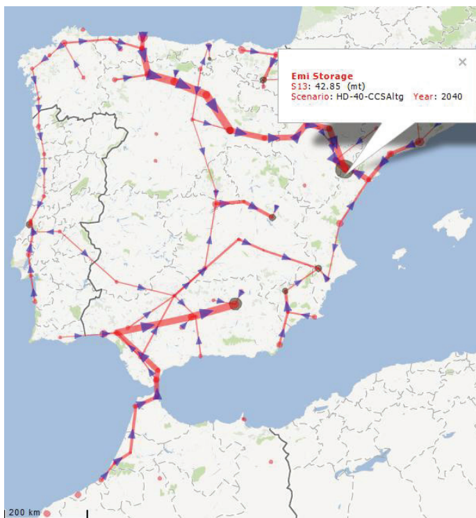
Figure 6 - CO 2 fluxes in Morocco, Portugal and Spain in 2040, assuming a high development of the demand for energy services, 40% emission reduction in 2050 and the need to follow the existing natural gas pipeline network.
