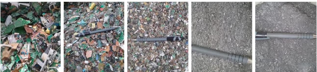
**Figure 2. WPCBs samples (raw material, -30 mm, -10 mm, -2 mm and -750 μm, from left to right).**
