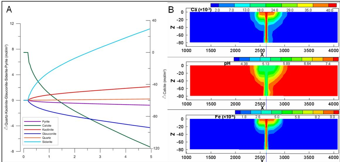
Figure 4 Evolution of mineral phases during  $\text{CO}_2$  ingress in the Albian formation (at the top of the leaking well) during  $\text{CO}_2$  leakage (A), aqueous concentrations (Ca, Fe in  $\text{mol/kgw}$ ) and pH in the Albian formation after 5 years (B)
