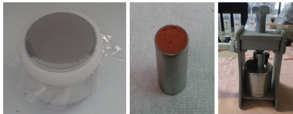
Figure 8. Sample prepared as a cup with film (left) or with a press, without film (centre) and press (right).
