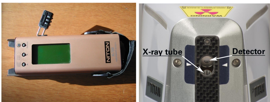
Figure 1. An early radioactive source portable X-ray fluorescence spectroscopy (pXRF) spectrometer (XLt723KWY), and the front part of a modern instrument (image courtesy of Bruker).
