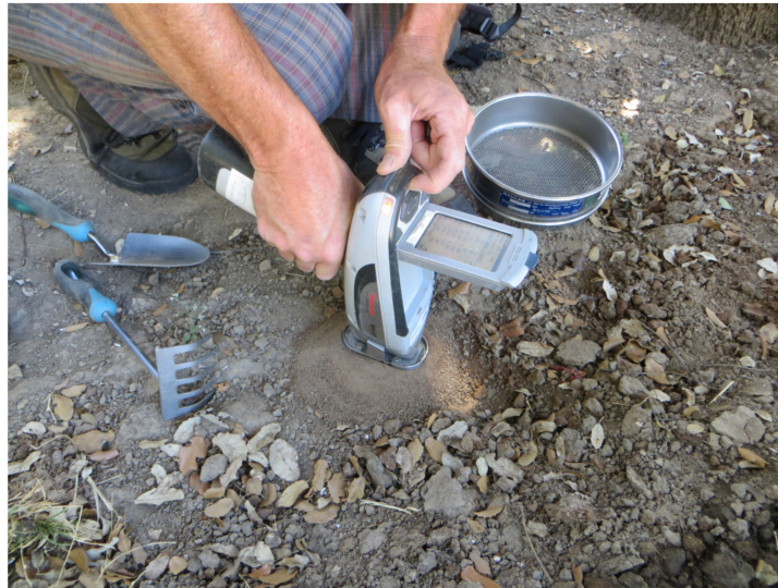
Figure 2. A modern tube-type pXRF spectrometer in on-site operation for a soil survey. The sample preparation procedure used here comprises a dry sieving to 2 mm, manual homogenisation of the sieved fraction, and light compaction by the shovel back. Sampling depth depends on the local soil profile and of the purposes of the study. Gravel and vegetal debris are removed by hand before sieving.
