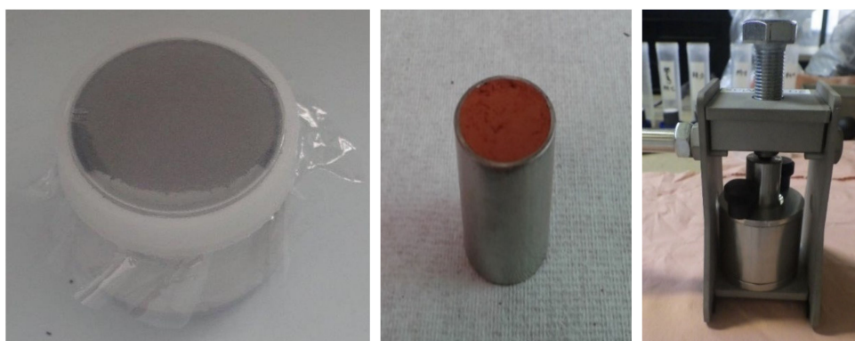
Figure 8. Sample prepared as a cup with film (left) or with a press, without film (centre) and press (right).
