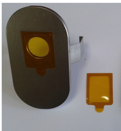
Figure 5. Protective shield of a Niton XL3t spectrometer.
