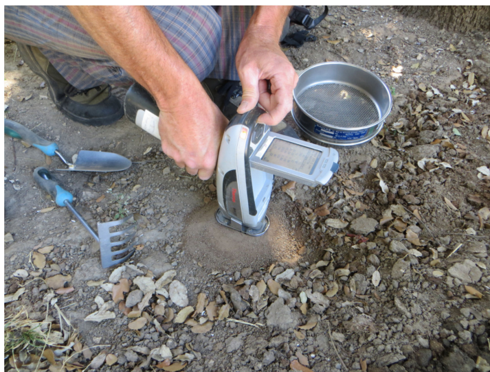
Figure 2. A modern tube-type pXRF spectrometer in on-site operation for a soil survey. The sample preparation procedure used here comprises a dry sieving to 2 mm, manual homogenisation of the sieved fraction, and light compaction by the shovel back. Sampling depth depends on the local soil profile and of the purposes of the study. Gravel and vegetal debris are removed by hand before sieving.
