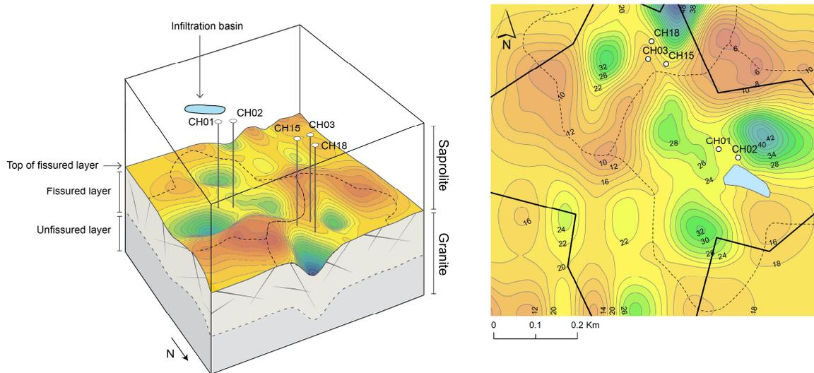
Figure 1: Topography of the transmissive bedrock interface interpreted from Electrical Resistivity Tomography profiles
