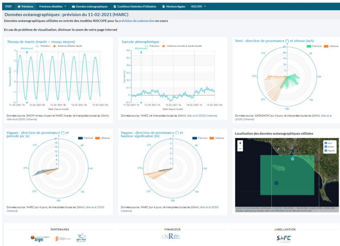
Figure A7. Screen capture of the FEWS webpage showing the forcing conditions X (here, X = X_{MARC} ). The forcing conditions in orange correspond to the last major flooding event (10 March 2008, Windstorm Johanna).
