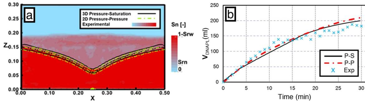
Figure 1. Simultaneous representation of experimental measurements and two simulation approaches for the 150 ml.min<sup>-1</sup> flowrate for: (a) distribution of water and DNAPL at the end of pumping scenario and (b) temporal evolution of the retrieved DNAPL
