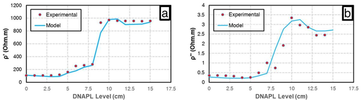
Figure 2. Simultaneous results of complex resistivity evolution through the fill-up scenario for an electrical injection/potential configuration at the bottom part of the domain: (a) in-phase resistivity and (b) quadrature resistivity
