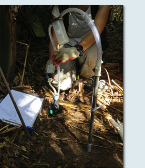
Measurement of radon 222 content in soil, to locate the zones affected by advective gas transfers that usually coincide vertically in hydraulically active fracture zones (B)
