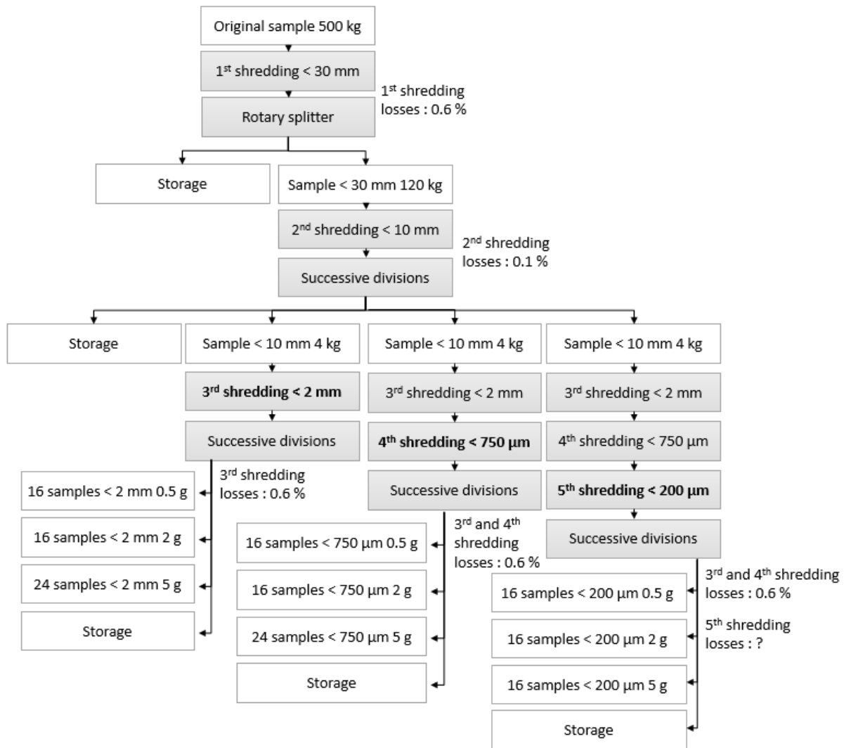
588 Figure 1: Sampling and shredding procedure.
