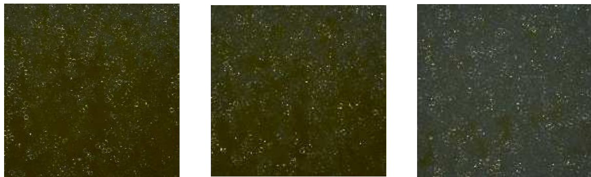
Figure 6: Images taken during (a) injection at 12 mL/min and (b) pumping at 6 mL/min of oil inside 1 mm glass beads initially saturated with ethanol. As oil is being injected, a sharp horizontal interface is being pushed in. On the contrary, when oil is being pumped, viscous fingers appear and trap the oil ganglia
