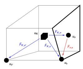
**Fig. 3** Matrix fluxes (*in blue*) and fracture fluxes (*in red*) inside a cell K with a fracture face  $\sigma$  (*in bold*). The matrix fluxes  $F_{K,\nu}$  connect the cell K to its nodes and fracture faces  $\nu \in \mathcal{V}_K \cup \mathcal{F}_{\Gamma,K}$ . The fracture fluxes  $F_{\sigma,\mathbf{s}}$  connect the face  $\sigma$  to the nodes  $\mathbf{s} \in \mathcal{V}_{\sigma}$  of  $\sigma$
