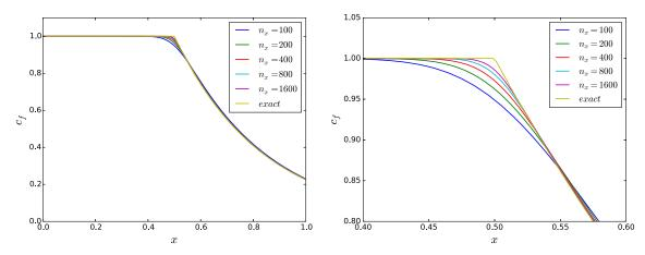
Fig. 7 Left: analytical solution and numerical solutions along the fracture at time  $t_f$  with  $n_x = 100, 200, 400, 800, 1600$ . Right: zoom view of left figure around x = 0.5
