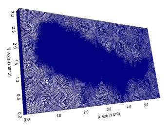
**Fig. 17** Prismatic mesh of the domain  $\Omega$  defined by the tensor product of a vertical 1D uniform mesh with a 2D triangular mesh
