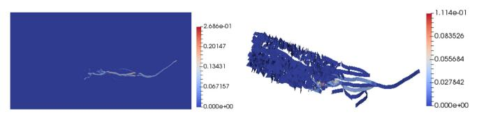
Fig. 22 Tracer concentration at final time in the matrix domain (left) and in the fracture network (right)
