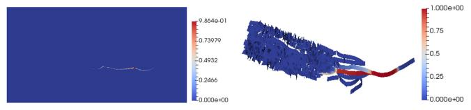
Fig. 21 Tracer concentration after 1 year of injection in the matrix domain (left) and in the fracture network (right)
