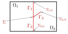
**Fig. 1** Example of a 2D domain with three intersecting fractures  $\Gamma_1$ ,  $\Gamma_2$ ,  $\Gamma_3$  and two connected components  $\Omega_1$ ,  $\Omega_2$
