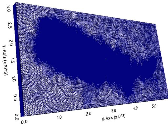
**Fig. 17** Prismatic mesh of the domain  $\Omega$  defined by the tensor product of a vertical 1D uniform mesh with a 2D triangular mesh
