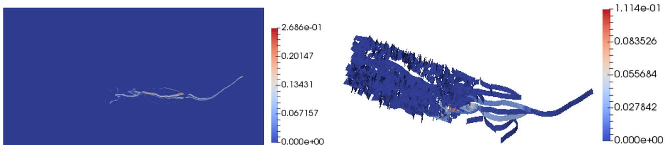
**Fig. 22** Tracer concentration at final time in the matrix domain (*left*) and in the fracture network (*right*)
