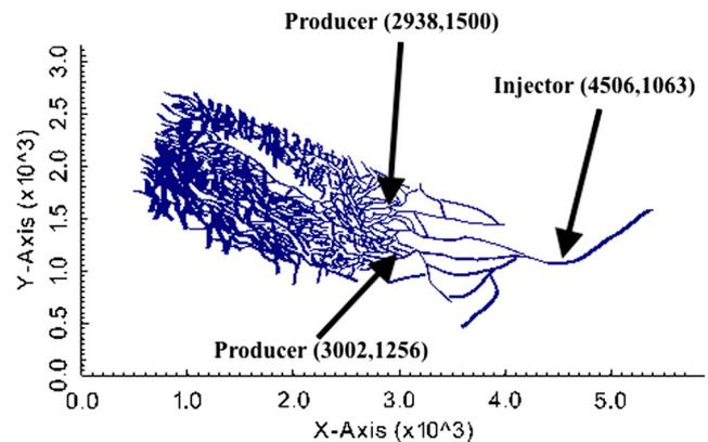
**Fig. 18** Fracture network showing the location of the single injection well and of the two production wells
