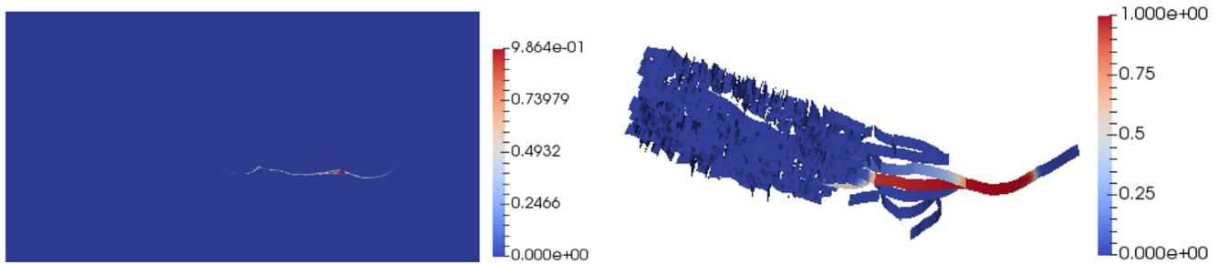
**Fig. 21** Tracer concentration after 1 year of injection in the matrix domain (*left*) and in the fracture network (*right*)
