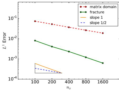
**Fig. 8** Relative  $L^1$  errors and references in the matrix domain and in the fracture at time  $t_f$  between the analytical solution and the numerical solutions as a function of the grid size  $n_x = 100, 200, 400, 800, 1600$
