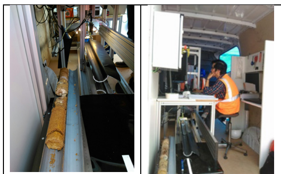
Figure 4: SOLSA core-scanner in a minivan (note that the XRF spectrometer was not mounted for security reasons).
