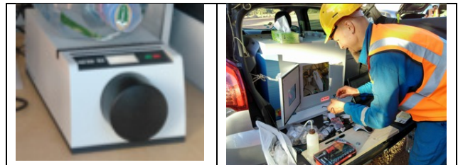
Figure 6. Micronizer, Retsch (BRGM) for fast milling of homogenous powders from the region of interest, drill muds & dusts.
