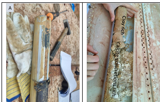
Figure 3. A. split liner showing bursting of rubber band, a result of swelling pressure due to clay minerals in marls, B. Calcite concretion-hosting marls.
